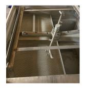
TURN THE BLUE VALVE TO THE LEFT. BE SURE TO TURN IT TIGHT. THIS WILL DRAIN THE WATER
